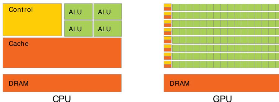
Figure 3: CPU design vs. GPU design [22, p. 3]
