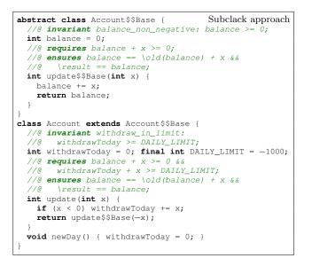
Figure 5: Composition of features *Base* and *DailyLimit* with the Subclack approach.
