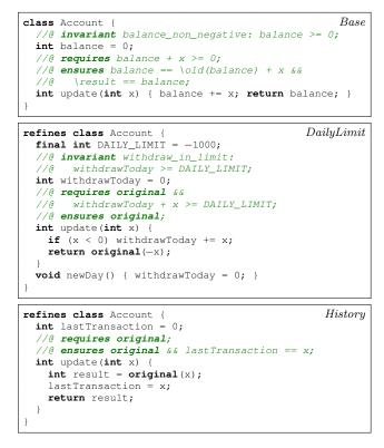
Figure 3: In explicit contract refinement, contracts can be defined for methods and method refinements; contracts for method refinements can refer to the original precondition or postcondition.
