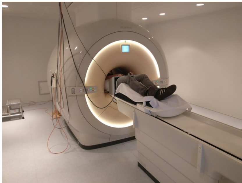
Figure 2.9: Participant in our fMRI scanner. Participants can view stimuli on a small plastic screen via a mirror on the head coil (cf. Figure 3.3). Participants respond to tasks with fMRI-compatible two-button response device.
