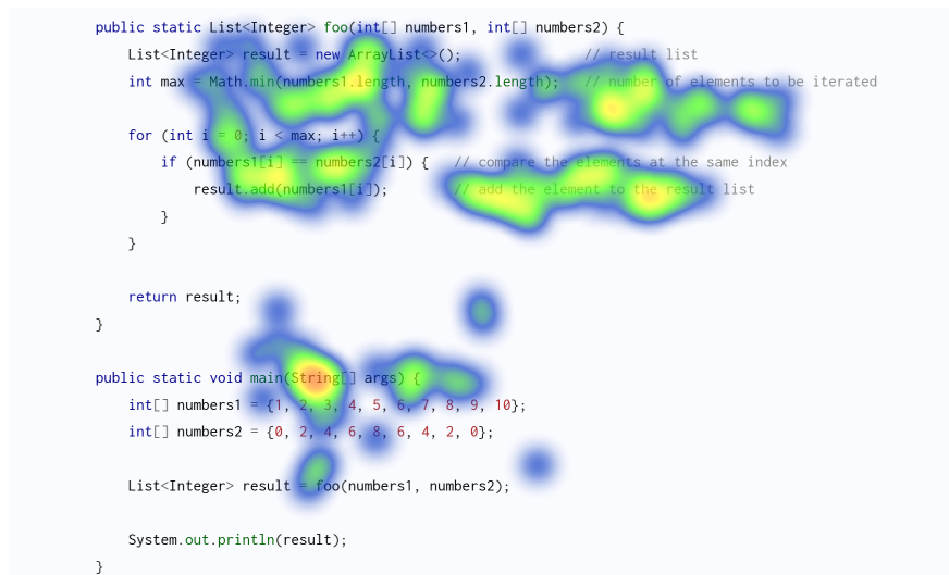
Figure 5.5: Example heatmap of eye fixations on a code snippet. The color intensity represents the fixation density, with warmer colors indicating higher fixation frequency.
