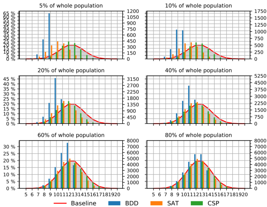
Figure A.21: Comparison of the cardinal distribution, for the sampling results of the mandatory and optional feature model with 20 configuration options. Shown are 6 subsets of sampled configurations in relation to the whole population. The appearance of a specific number of selected configuration options are shown with a bar indicating the percentual number of configurations with this length, within the sampled subset. On the opposite side we show the absolute number of configurations, with this length within the sampled subset.
