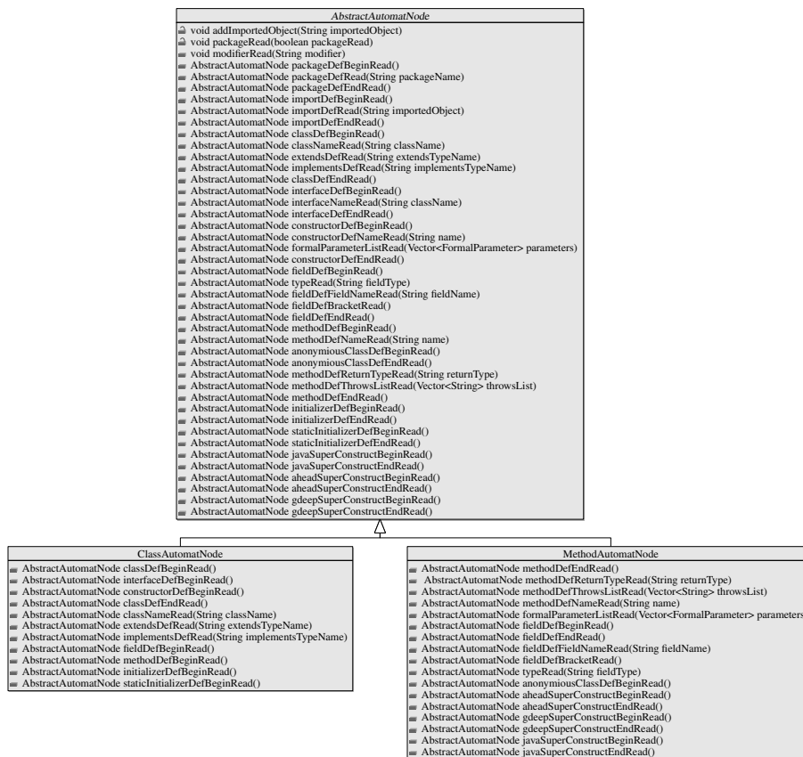
Figure A.1.: The extract of the UML model of the state machines' classes
