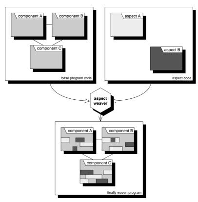
Figure 2.11 illustrates the weaving of two aspects into a base program consisting of three components.
