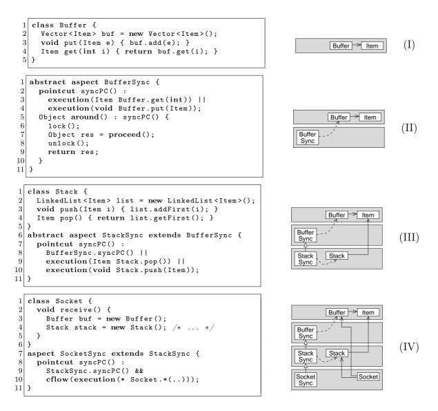
Figure 6.1: Four steps in the evolution of a program using AFMs.
