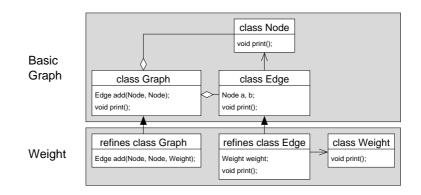
Figure 2.4: Collaboration-based design of a graph implementation.
