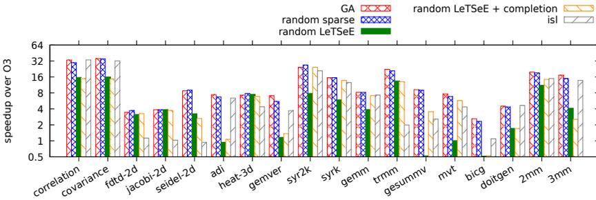
Fig. 7. Speedups over plain O3 reached by different configurations. The baseline is O3.
