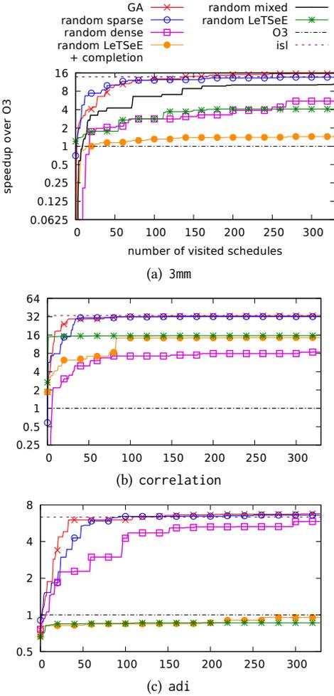
Fig. 5. Convergence rate of different configurations of iterative optimization. The  $x$ -axis shows the number of schedules already visited. The  $y$ -axis shows speedup over O3. For convenience, also the speedup reached by the isl-scheduler is shown. Only every 20th data point is plotted.
