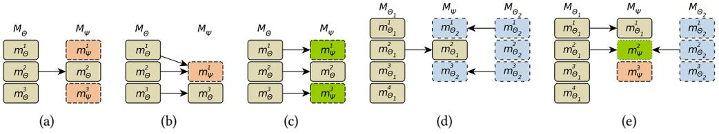
Fig. 2. Illustration of schedule mutation and crossover operators: (a) dimension replacement; (b) prefix replacement; (c) generator coefficient replacement; (d) row-based crossover; (e) geometric crossover
