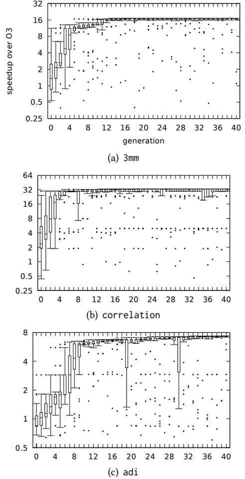
Fig. 6. Box plots showing the distribution of performance within the generations of the GA. The data are from Exp. 3. The length of the whiskers is 1.5 times the interquartile range. The whiskers may have been truncated to remain within the data set's range. The dots are outliers beyond the range of the whiskers.
