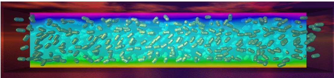
**Figure 4.10.:** Interactive visualization of a coupled WALBERLA and *pe* simulation. Several capsules are located inside a box filled with liquid, at top and bottom opposing flows exist. The velocity in x direction is visualized [64].
