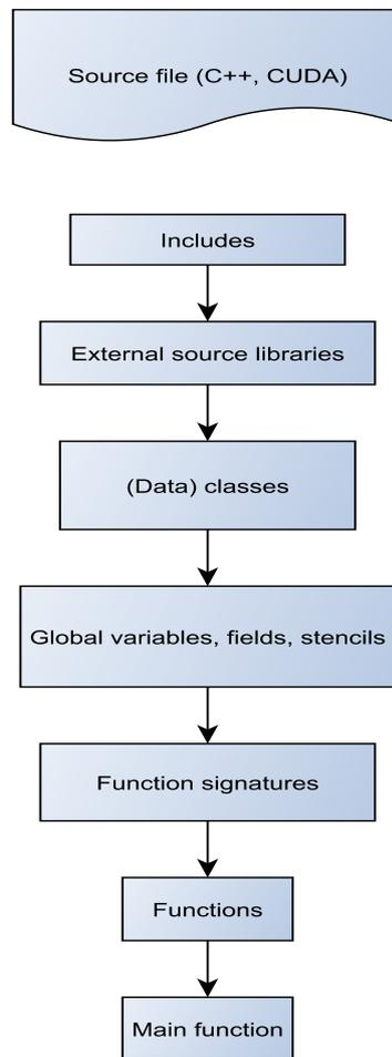
Figure 6.6.: Structure of the pretty-printed source file.
