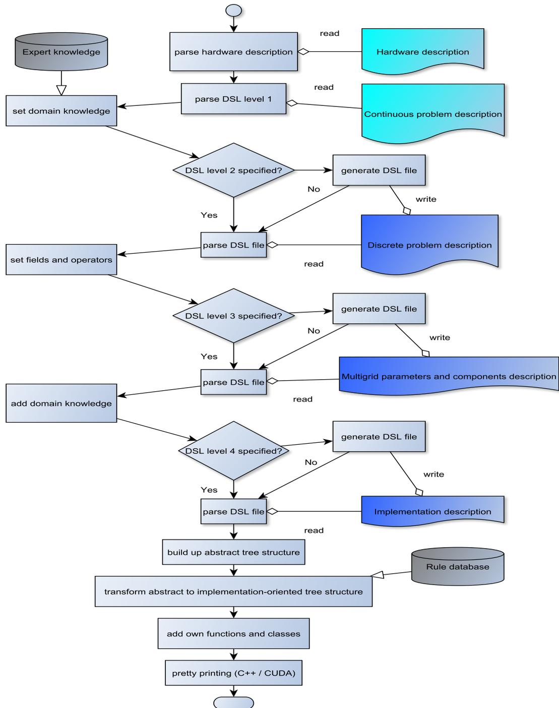
**Figure 6.5.:** General structure of Scala prototype. DSL descriptions on different levels are parsed, transformed into an implementation-oriented representation, and then pretty-printed to C++ or CUDA source code.
