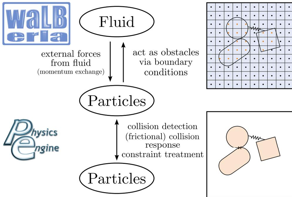
**Figure 4.9.:** Illustration of the four-way coupling of the WALBERLA LBM fluid solver and *pe* rigid body physics engine [44].
