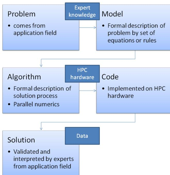
**Figure 3.3.:** Schematic workflow for a prototypical CSE application.
