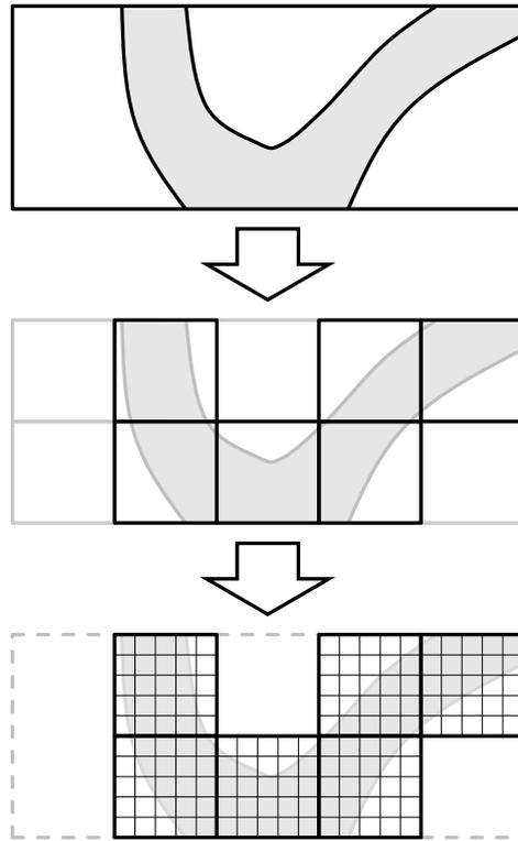
**Figure 4.3.:** Two-stage domain partitioning: block division and subsequent grid generation [30].
