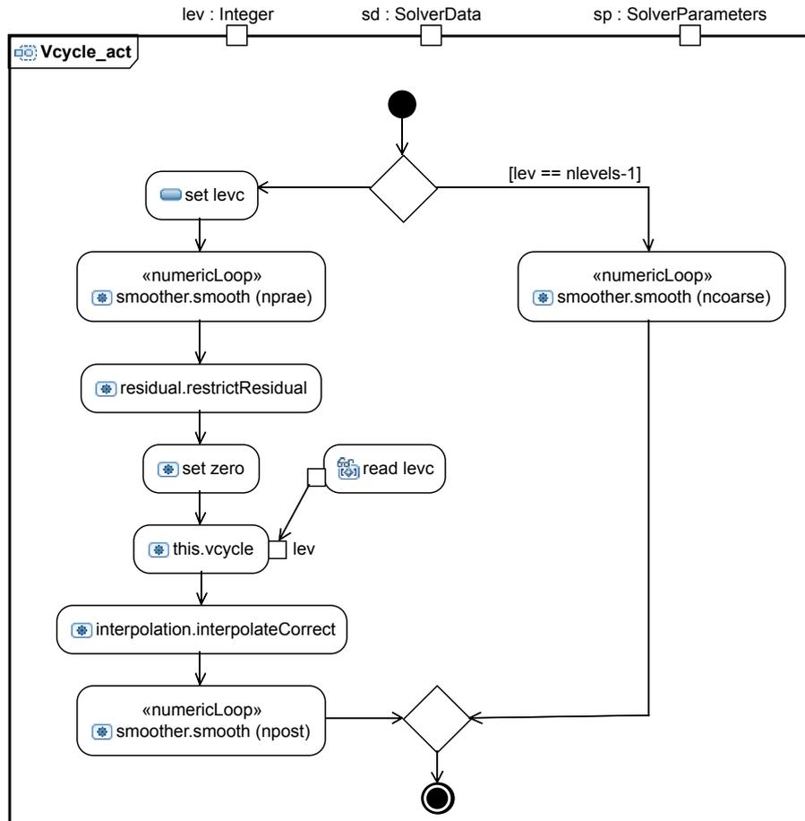
Figure 5.2.: UML activity diagram representing an abstract implementation of the V-cycle algorithm 5.1 [24].
