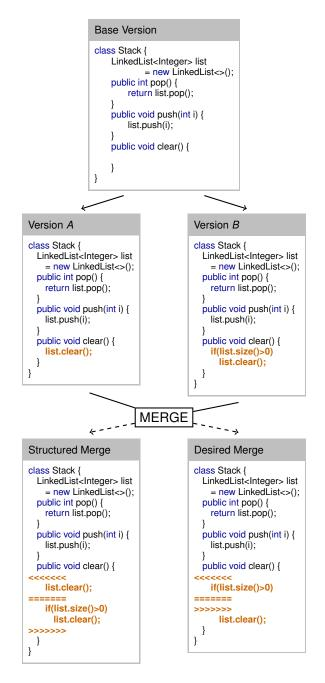
Figure 3. Shifted code example: Stack.java
