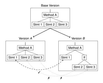
Figure 1. Top-down, level-wise AST matching (*Stmt 1* can be matched ( $\checkmark$ ); *Stmt 2* and *Stmt 3* can not be matched ( $\checkmark$ ) as they are not at the same level)
