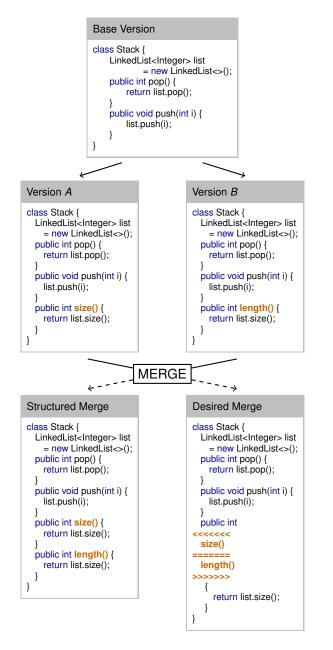
Figure 2. Method renaming example: Stack.java
